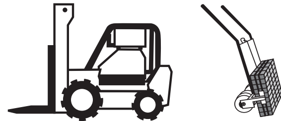
Figure 21. Fork lift and paver cart used to bring pavers to laying face.
